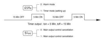
When using MOC '1', main output will be OFF automatically as timer is ON. If using MOC function, you can effectively use timer output as a defrosting function.
