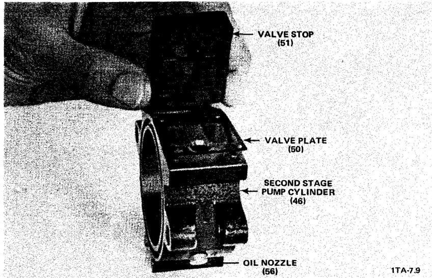
**NOTE:** The valve plate (50) on the D30A/D60A/D90A pump models has four tabs rather than two.
