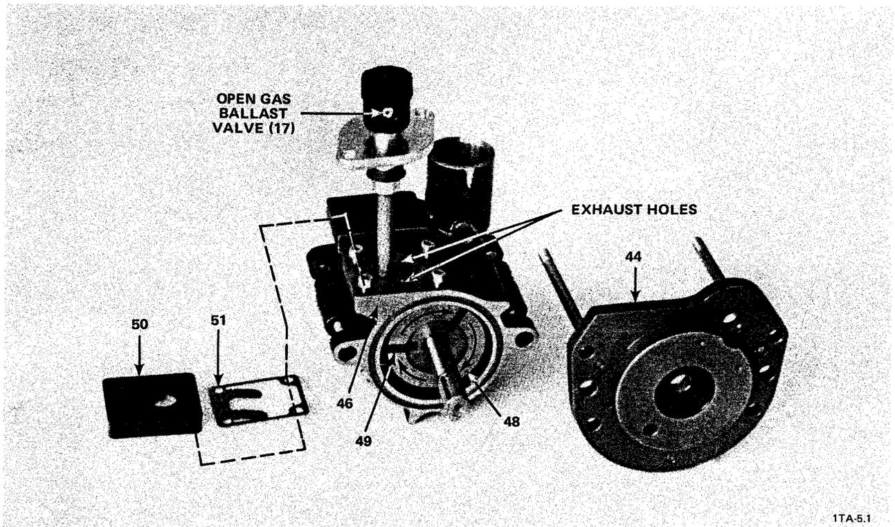
**NOTE:** This photograph is for illustration purposes only. When assembled, the cap end of the gas ballast valve (17) is attached outside the top of the oil casing (12) (see Figure 1-1), and an oil filter (35) and other parts fit around the valve (17) stem (see Figure 5-10B).
