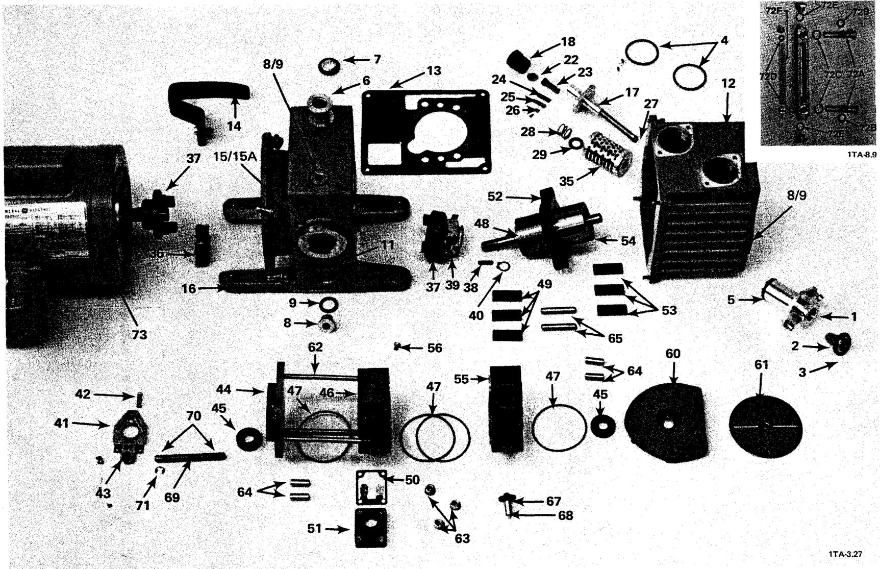
Figure 7-1. Disassembled Pump (D2A Pump Model Shown)
